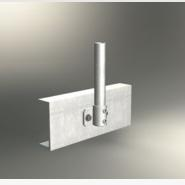
**F2 - Face Mount (2 Fixings)** Concrete - using M12 x 100mm galvanized screwbolts Steel - using M16 hi-tensile galvanized bolts
