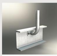
C13 - Channel Mount (2 Fixings) 130 mm Offset Steel - using M16 hi-tensile galvanized bolts
