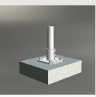
**T4 - Top Mount (4 Fixings)** Concrete - using M12 x 100mm galvanized screwbolts Steel - using M16 hi-tensile galvanized bolts
