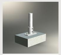
**T2 - Top Mount (2 Fixings)** Concrete - using M12 x 100mm galvanized screwbolts Steel - using M16 hi-tensile galvanized bolts
