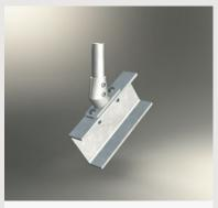
AM - Angle Mount (2 Fixings) Concrete - using M12 x 100mm galvanized screwbolts Steel - using M16 hi-tensile galvanized bolts
