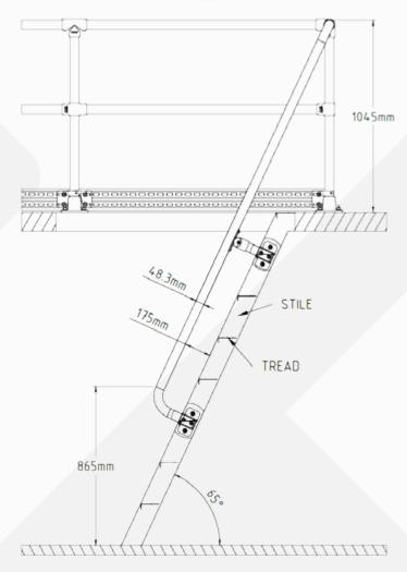
The section view above shows a custom height Assistrail AR10 system mounted onto a 65° ladder joining into Tuffrail TR25 on a platform above.
